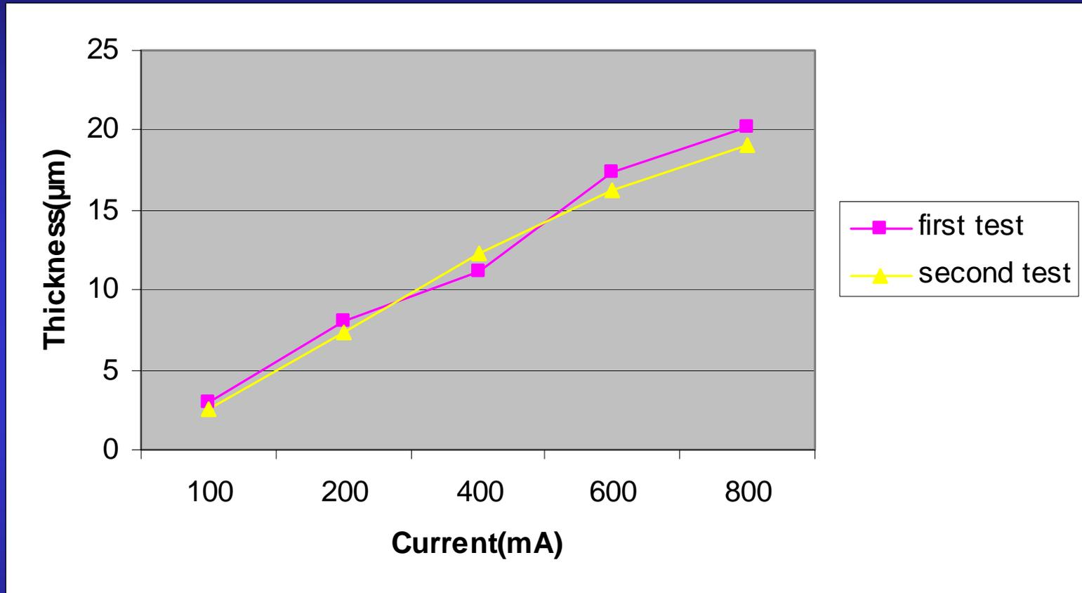
The deposition rate is proportional to the applied current, but too much current is responsible for a higher Sn roughness and also for a bad adhesion between Sn and Ag
