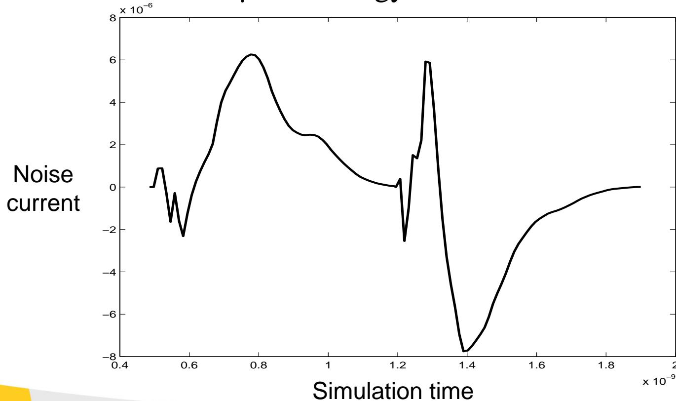
Total injection noise from capacitive coupling and impact ionization in a single inverter in the simulation.
