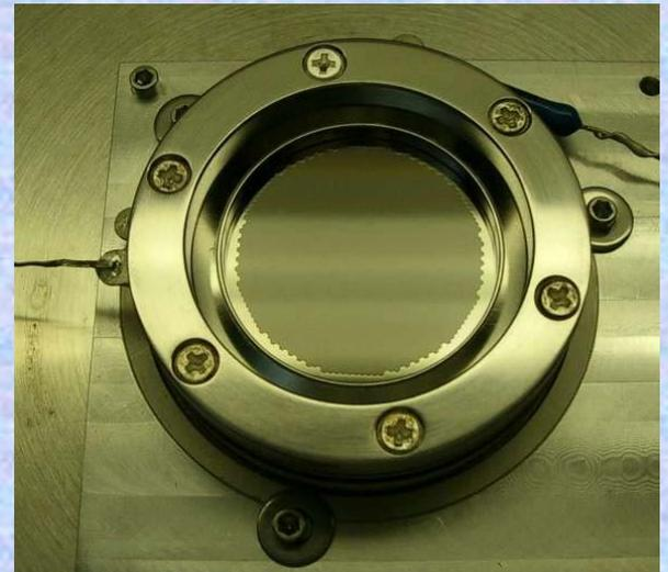
25mm cross delay line anode detector showing neutron sensitive MCPs
