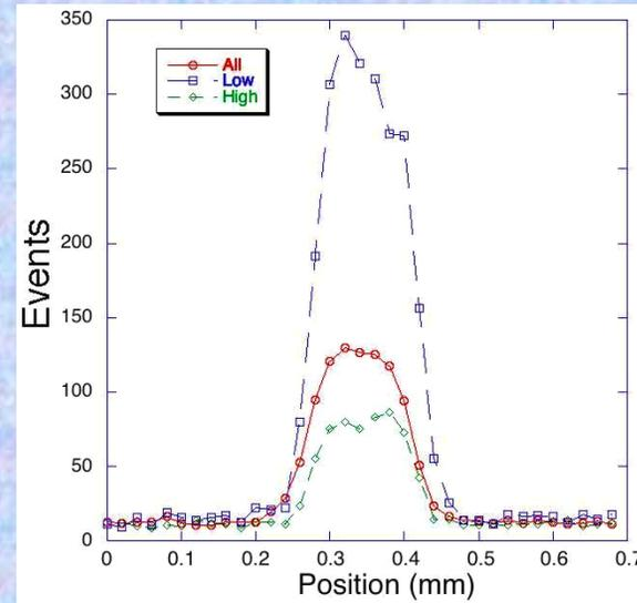
Image slice across one arm of the star pattern. Contrast is poor if all events, or only high amplitude events are used. Using only the low amplitude peak events gives a high contrast (30:1) image at the expense of some efficiency.
