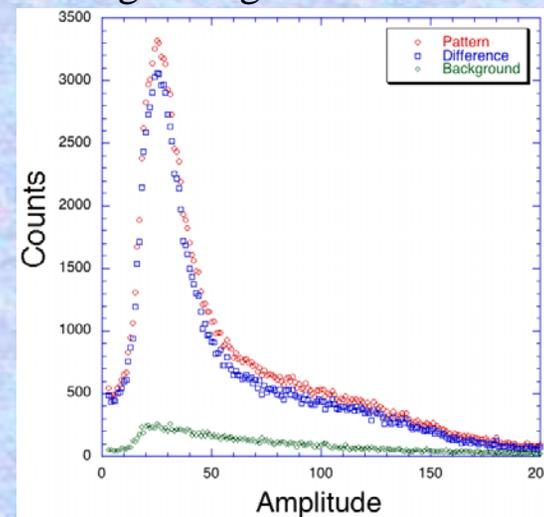
PHDs for through, and under mask. Neutron (alpha) events give high amplitudes.
