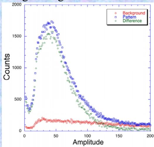
PHDs for through, and under mask, gammas dominate at high amplitudes
